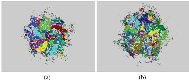
Fig. 12. (a) Burning cells in the SwirlH2 data at time step 1500 using a fuel consumption threshold of  $8.0 \text{ kg}_{\text{H}_2}/\text{m}^3 \text{ s}$ ; (b) Burning cells in the SwirlH2Fast data at threshold  $12.0 \text{ kg}_{\text{H}_2}/\text{m}^3 \text{ s}$ .
