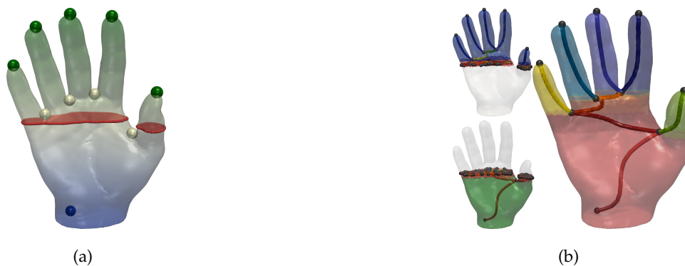
Figure 5.1 – Algorithm overview on the height function f of a volume \mathcal{M} with two threads. (a) Input scalar field f (color gradient) with its critical points (blue: min, white: saddle, green: max). The domain is split into two partitions \mathcal{P}_i and \mathcal{P}_j of roughly equal size corresponding to the pre-images of contiguous intervals \mathcal{I}_i and \mathcal{I}_j of f(\mathcal{M}) . The interface level-set between such two partitions is shown in red. (b) The augmented contour trees \mathcal{C}(f)_i (top) and \mathcal{C}(f)_j (bottom) are constructed in parallel for each partition. These local trees can be easily and efficiently stitched together to form the output augmented contour tree (right).
