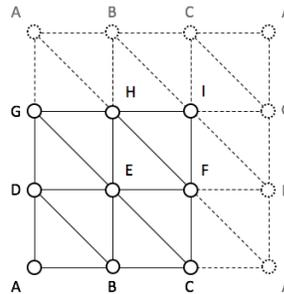
**Fig. 6** The periodic triangulation in 2D is accomplished by adding the dashed edges and triangles to the triangulation shown with solid edges.
