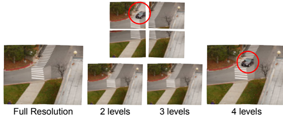
Figure 1: An example case where a deep hierarchy for Hierarchical Graph Cuts produces poor results. A car that appears in only one of the input images (top) causes a region with high energy which a pixel based energy will avoid. The results for up to 3 levels are good. At 4 levels, in the coarse solution, the car is small enough for the seam to pass through it. The dilatation parameter (10 pixels in the typical case) is not large enough to exit this local minima in the refinement stages.
