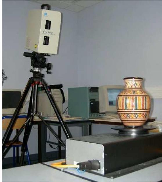
Figure 2.6 – Lab's Minolta VI-300 laser range scanner.
